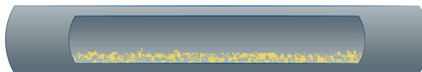
Dust particles can build up when air velocity is less than 3500 feet per minute.
