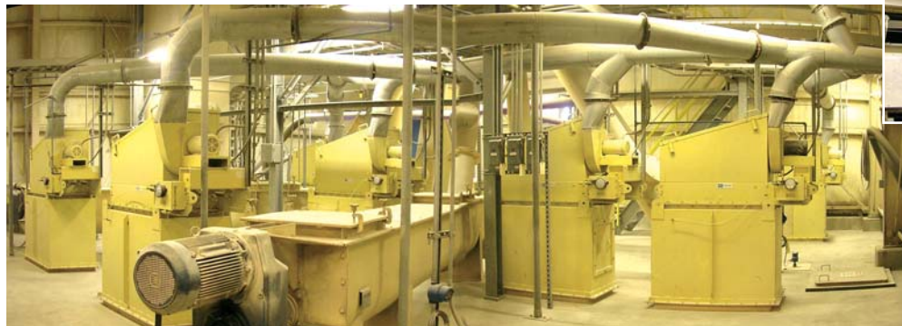
Dalamatric insertable collectors (the tops are slanted) are venting each raw material silo in this room at the top of a batch house. Clean-side access for service eliminates the need for OSHA “confined space” entry permits and procedures.
