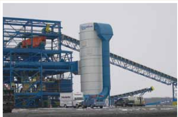
780LP12 at coal classifying plant (75,000 cfm)
